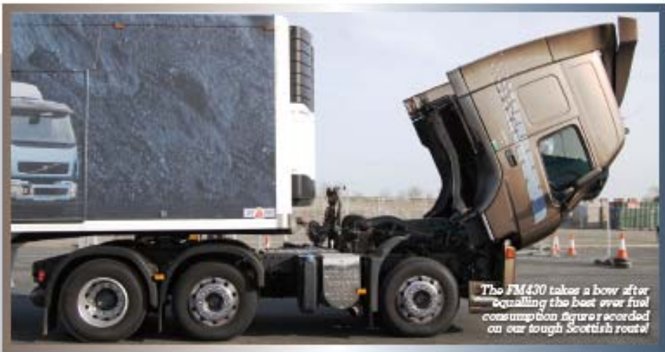
Fuel tank cleverly incorporates two recessed safety steps.
