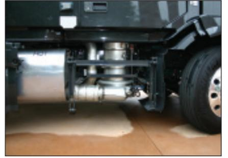
**TAKING A PEAK:** The SCR catalyst is located on the passenger side of the truck, but hidden from sight by the side fairings.
