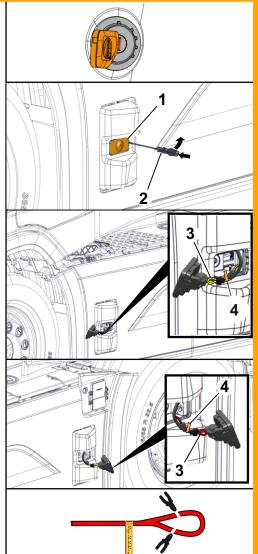
Cut the emergency cut-off loop on each side of the loop to disconnect the traction voltage supply from the traction batteries.
