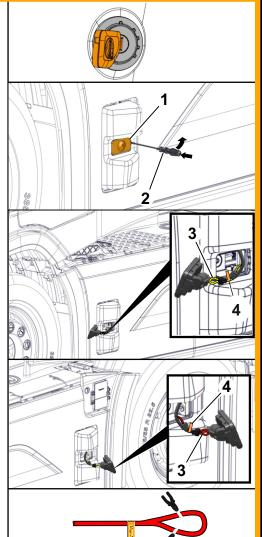
Cut the emergency cut-off loop on each side of the loop to disconnect the traction voltage supply from the traction batteries.
