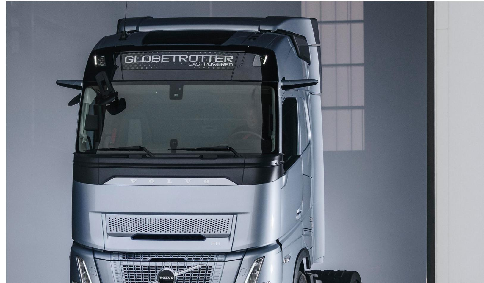
correctly adjusted to gain full potential. Recent findings at Volvo Trucks indicate that the correct setting can save between 2–6% in fuel. Ideally, the roof spoiler should be factory fitted from the start.
